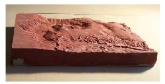
Fig. 5: Negative mould covered with caoutchouc.
