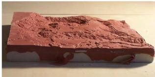
Fig. 2: Negative step model covered by red caoutchouc.
