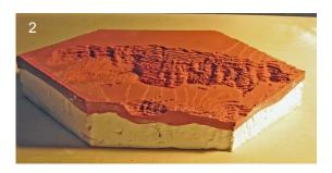
Make a negativmodel from the stepmodel with liquid silicon - rubber
