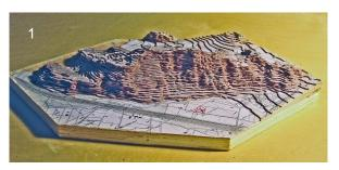
Put the cutted parts to a exat stepmodel, using the contourlines and the coordinatenet for an exact assembly
